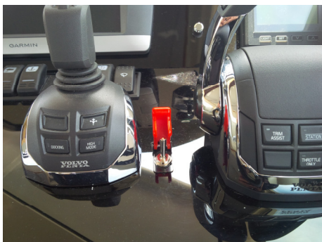
Fuel emergency shut-off -Valves CLOSED position-
