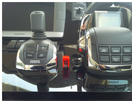
Fuel emergency shut-off -Valves OPEN position-
